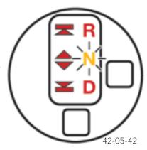
This display is illuminated when the transmission is in the *mechanical emergency operation* (with forward movement). The R and N illumination will remain on and all of the arrows along with the D position indicator will flash at a frequency 1.5 Hz.
